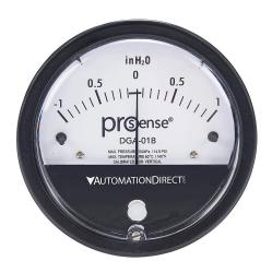
ProSense differential pressure gauge, 4in dial diameter, -1.0 to +1.0in of water column, black die-cast aluminum case, aluminum and silicone rubber wetted parts, (2) high and (2) low 1/8in female NPT process connection, panel or surface mount.
