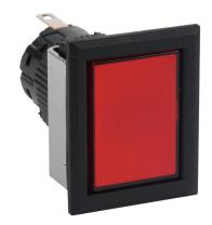
Fuji Electric LED indicating light, permanent light function, IP65, 16mm, red, 28mm, rectangular, plastic base, plastic bezel, 24 VAC/VDC, full voltage.
