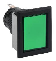
Fuji Electric LED indicating light, permanent light function, IP65, 16mm, green, 28mm, rectangular, plastic base, plastic bezel, 24 VAC/VDC, full voltage.
