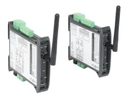
Define Instruments Twin Link series wireless signal transmitter/ receiver, isolated, Input: 2-channel, current/bipolar voltage/freq/ potentiometer/thermocouple/RTD, deg F or deg C, Output: 2-channel, loop powered current, ZigBee: 2.4 GHz, 9-36 VDC operating voltage.
