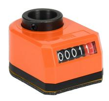
Elesa position indicator, 5-digit mechanical, inclined lower, 0001.0 counts per revolution, counter clockwise, 20mm mounting hole size, IP65.
