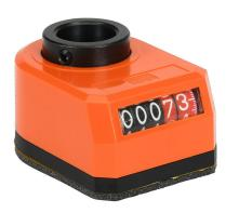
Elesa position indicator, 5-digit mechanical, inclined lower, 000.50 counts per revolution, counter clockwise, 3/4in mounting hole size, IP65.
