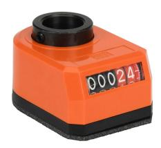
Elesa position indicator, 5-digit mechanical, inclined lower, 000.50 counts per revolution, clockwise, 3/4in mounting hole size, IP65.
