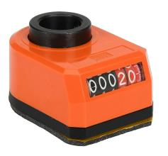
Elesa position indicator, 5-digit mechanical, inclined lower, 000.20 counts per revolution, counter clockwise, 3/4in mounting hole size, IP65.
