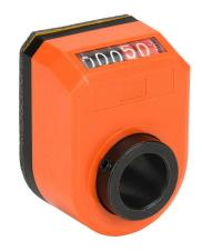
Elesa position indicator, 5-digit mechanical, inclined upper, 000.50 counts per revolution, clockwise, 3/4in mounting hole size, IP65.
