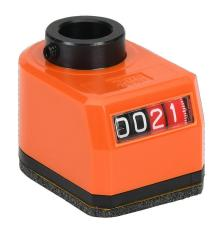
Elesa position indicator, 4-digit mechanical, inclined lower, 00.20 counts per revolution, counter clockwise, 1/2in mounting hole size, IP65.
