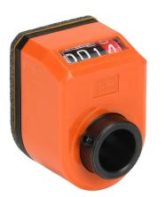
Elesa position indicator, 4-digit mechanical, inclined upper, 001.0 counts per revolution, clockwise, 14mm mounting hole size, IP65.
