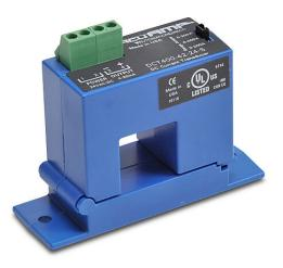
AcuAMP DC current transducer, split core, 0-200, 0-300, or 0-400A selectable sensing range, 4-20 mA output.
