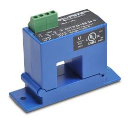
AcuAMP DC current transducer, split core, bi-directional 0-300A sensing range, bipolar +/- 0-10 VDC output.
