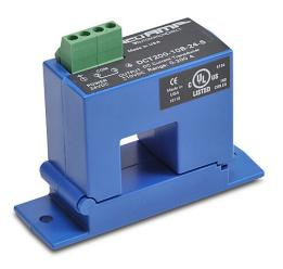
AcuAMP DC current transducer, split core, bi-directional 0-200A sensing range, bipolar +/- 0-10 VDC output.
