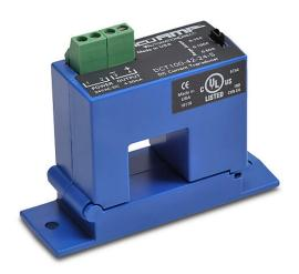
AcuAMP DC current transducer, split core, 0-50, 0-75, or 0-100A selectable sensing range, 4-20mA output.
