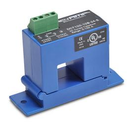
AcuAMP DC current transducer, split core, bi-directional 0-100A sensing range, bipolar +/- 0-10 VDC output.
