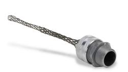
Bryant deluxe strain relief grip, accepts cable diameter size 0.62 to 0.75in, straight 1in NPT male thread fitting, stainless steel mesh, 6.11in length, indoor and outdoor applications.
