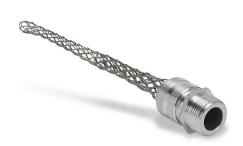
Bryant deluxe strain relief grip, accepts cable diameter size 0.5 to 0.62in, straight 3/4in NPT male thread fitting, stainless steel mesh, 4.71in length, indoor and outdoor applications.
