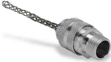
Bryant deluxe strain relief grip, accepts cable diameter size 0.18 to 0.25in, straight 1/2in NPT male thread fitting, stainless steel mesh, 2.44in length, indoor and outdoor applications.
