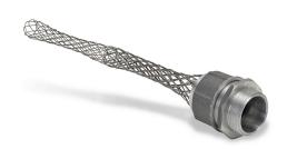
Bryant deluxe strain relief grip, accepts cable diameter size 1.56 to 1.68in, straight 2in NPT male thread fitting, stainless steel mesh, 10in length, indoor and outdoor applications.
