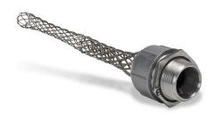
Bryant deluxe strain relief grip, accepts cable diameter size 1.12 to 1.25in, straight 1-1/4in NPT male thread fitting, stainless steel mesh, 6.04in length, indoor and outdoor applications.
