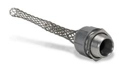
Bryant deluxe strain relief grip, accepts cable diameter size 1.12 to 1.25in, straight 1-1/4in NPT male thread fitting, stainless steel mesh, 6.04in length, indoor and outdoor applications.
