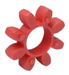
SureMotion drive coupling spider, jaw type, size 65, polyurethane, 98A durometer. For use with DC-JAC65 series hubs.
