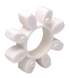
SureMotion drive coupling spider, jaw type, size 65, polyurethane, 92A durometer. For use with DC-JAC65 series hubs.
