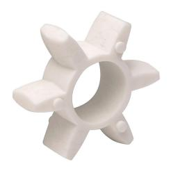
SureMotion drive coupling spider, jaw type, size 40, polyurethane, 92A durometer. For use with DC-JAC40 series hubs.
