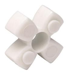
SureMotion drive coupling spider, jaw type, size 30, polyurethane, 92A durometer. For use with DC-JAC30 series hubs.
