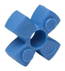
SureMotion drive coupling spider, jaw type, size 30, polyurethane, 80A durometer. For use with DC-JAC30 series hubs.
