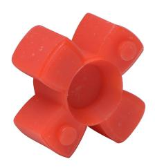
SureMotion drive coupling spider, jaw type, size 20, polyurethane, 98A durometer. For use with DC-JAC20 series hubs.
