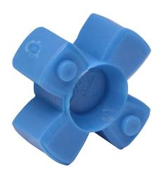
SureMotion drive coupling spider, jaw type, size 20, polyurethane, 80A durometer. For use with DC-JAC20 series hubs.
