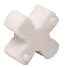
SureMotion drive coupling spider, jaw type, size 14, polyurethane, 92A durometer. For use with DC-JAC14 series hubs.
