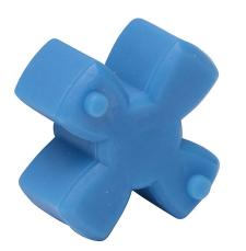
SureMotion drive coupling spider, jaw type, size 14, polyurethane, 80A durometer. For use with DC-JAC14 series hubs.
