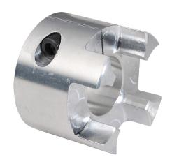
SureMotion drive coupling hub, jaw type, aluminum alloy, clamp, size 65, 32mm bore. Requires DC-JS65 series spiders.
