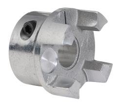
SureMotion drive coupling hub, jaw type, aluminum alloy, clamp, size 55, 3/4in bore. Requires DC-JS55 series spiders.
