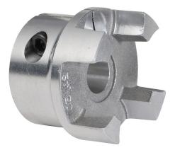
SureMotion drive coupling hub, jaw type, aluminum alloy, clamp, size 55, 5/8in bore. Requires DC-JS55 series spiders.
