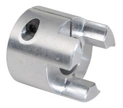
SureMotion drive coupling hub, jaw type, aluminum alloy, clamp, size 40, 3/4in bore. Requires DC-JS40 series spiders.
