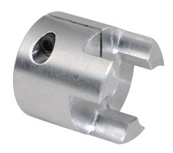
SureMotion drive coupling hub, jaw type, aluminum alloy, clamp, size 40, 5/8in bore. Requires DC-JS40 series spiders.
