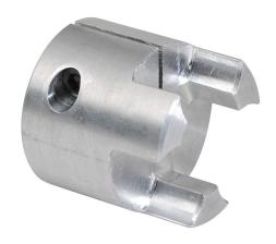
SureMotion drive coupling hub, jaw type, aluminum alloy, clamp, size 40, 8mm bore. Requires DC-JS40 series spiders.
