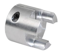
SureMotion drive coupling hub, jaw type, aluminum alloy, clamp, size 40, 3/8in bore. Requires DC-JS40 series spiders.
