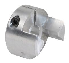
SureMotion drive coupling hub, jaw type, aluminum alloy, clamp, size 30, 10mm bore. Requires DC-JS30 series spiders.
