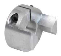
SureMotion drive coupling hub, jaw type, aluminum alloy, clamp, size 30, 1/2in bore. Requires DC-JS30 series spiders.
