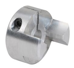
SureMotion drive coupling hub, jaw type, aluminum alloy, clamp, size 30, 8mm bore. Requires DC-JS30 series spiders.
