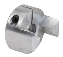
SureMotion drive coupling hub, jaw type, aluminum alloy, clamp, size 30, 3/8in bore. Requires DC-JS30 series spiders.
