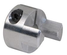
SureMotion drive coupling hub, jaw type, aluminum alloy, clamp, size 20, 1/4in bore. Requires DC-JS20 series spiders.
