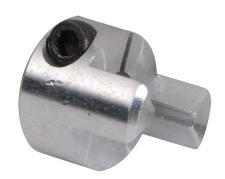
SureMotion drive coupling hub, jaw type, aluminum alloy, clamp, size 14, 6mm bore. Requires DC-JS14 series spiders.
