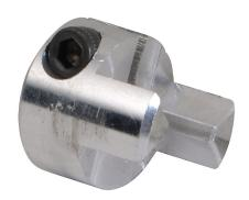
SureMotion drive coupling hub, jaw type, aluminum alloy, clamp, size 14, 5mm bore. Requires DC-JS14 series spiders.
