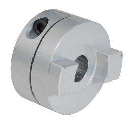
SureMotion drive coupling hub, Oldham, aluminum alloy, clamp, size 57, 16mm bore. Requires DC-DDS57 torque disc.
