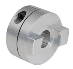
SureMotion drive coupling hub, Oldham, aluminum alloy, clamp, size 57, 3/4in bore. Requires DC-DDS57 torque disc.
