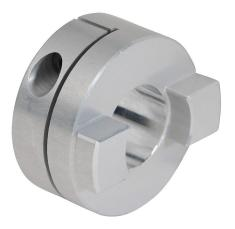
SureMotion drive coupling hub, Oldham, aluminum alloy, clamp, size 41, 3/4in bore. Requires DC-DDS41 torque disc.
