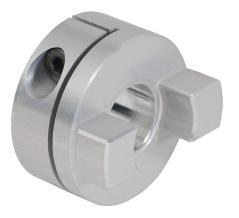
SureMotion drive coupling hub, Oldham, aluminum alloy, clamp, size 33, 14mm bore. Requires DC-DDS33 torque disc.
