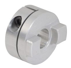
SureMotion drive coupling hub, Oldham, aluminum alloy, clamp, size 25, 3/8in bore. Requires DC-DDS25 torque disc.
