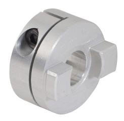
SureMotion drive coupling hub, Oldham, aluminum alloy, clamp, size 25, 3/8in bore. Requires DC-DDS25 torque disc.
