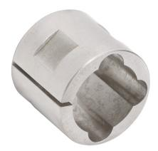
SureMotion bore reducer, clamping, stainless steel body, 7/8in outside diameter, 16mm inside diameter.
